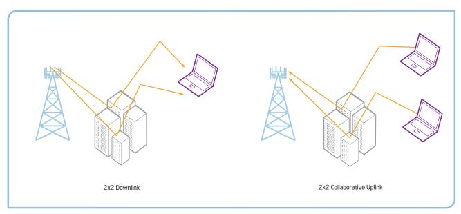
MIMO is a key enabler of WiMAX that exploits environmental phenomena such as multi-path propagation to increase data throughput and range.
