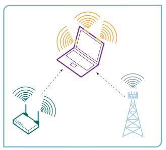
Innovative integrated antenna design enables both Wi-Fi and WiMAX to share antennas for platform-level noise mitigation
