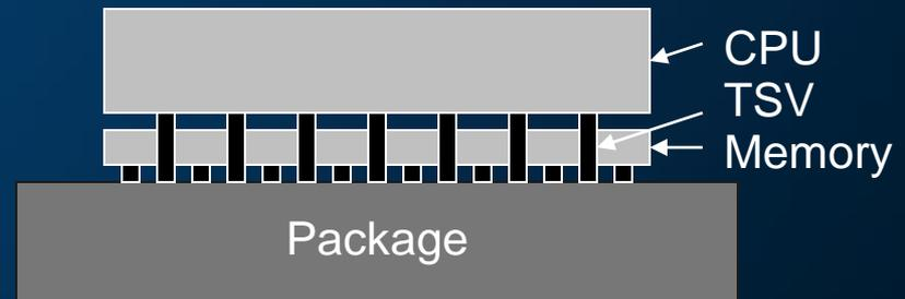
3-D chip stacking using through-silicon vias
