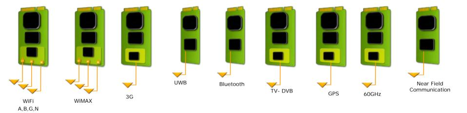
Poor analog and RF scaling do not prevent single chip integration but make it economically non viable. Digital cannot "wait" for analog die size reduction
