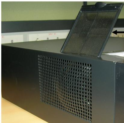
The dust filter can be removed and cleaned whenever it gets dirty.
