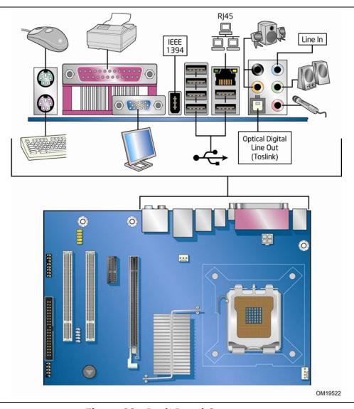
**Figure 28. Back Panel Connectors**
