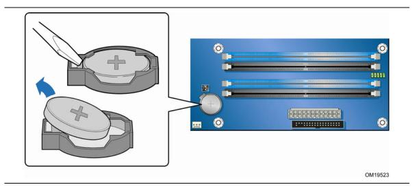
Figure 29. Removing the Battery
