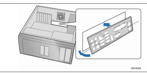
Figure 4. Installing the I/O Shield
