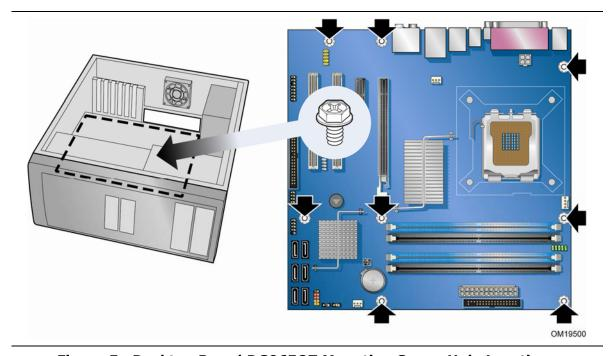
Figure 5. Desktop Board DG965OT Mounting Screw Hole Locations
