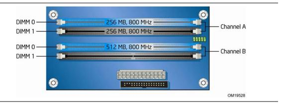
Figure 15. Dual Channel Memory Configuration Example 3
