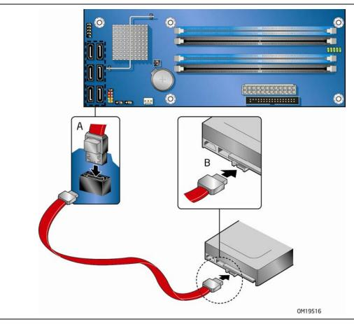
Figure 21. Connecting the Serial ATA Cable
