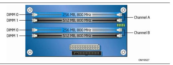
Figure 14. Dual Channel Memory Configuration Example 2
