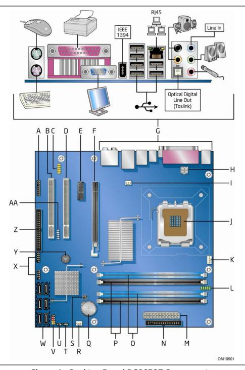
Figure 1. Desktop Board DG9650T Components
