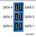
Figure 30. Original SATA Port Mapping for Desktop Board DG965OT
