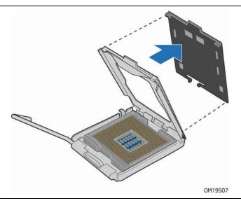
Figure 8. Remove the Protective Socket Cover
