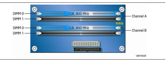
Figure 13. Dual Channel Memory Configuration Example 1
