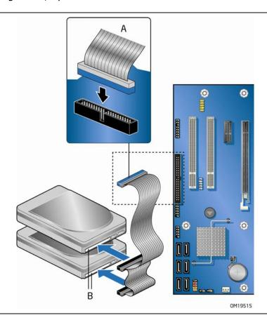
Figure 20. Connecting the IDE Cable
