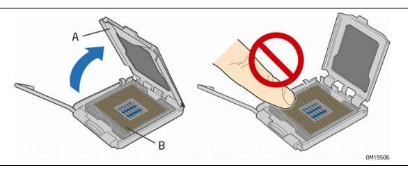
Figure 7. Lift the Load Plate
