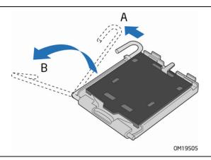
Figure 6. Lift Socket Lever
