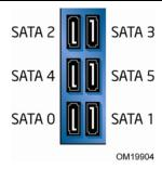
Figure 31. SATA Port Mapping for Desktop Board DG965OT After RAID is Enabled
