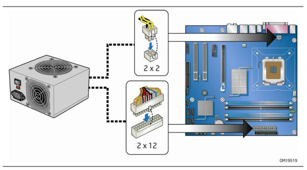
Figure 25. Connecting Power Supply Cables
