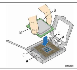
**Figure 10. Install the Processor**
