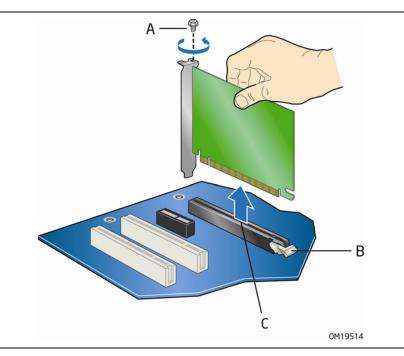
Figure 19. Removing a PCI Express x16 Card
