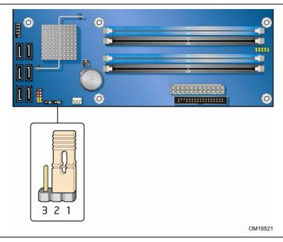
Figure 27. Location of the BIOS Configuration Jumper Block
