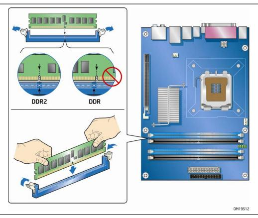
Figure 17. Installing a DIMM
