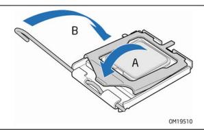
Figure 11. Close the Load Plate
