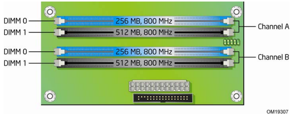
Figure 14. Dual Channel Memory Configuration Example 2
