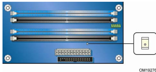
Figure 3. Location of Standby Power Indicator
