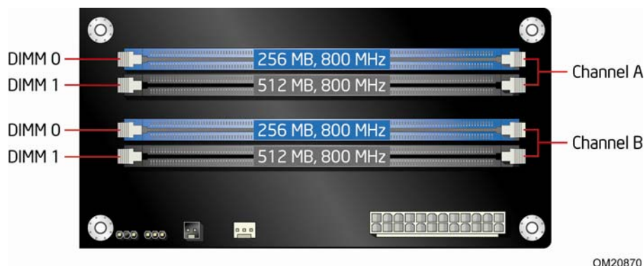
Figure 15. Dual Channel Memory Configuration with Four DIMMs
