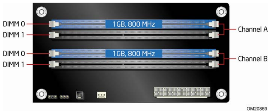
Figure 14. Dual Channel Memory Configuration with Two DIMMs
