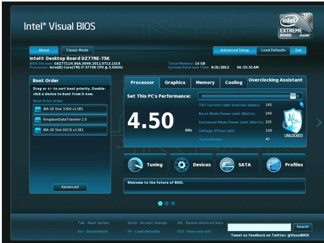
The Overclocking Assistant can be found on the home screen of the Visual BIOS setup. Note the 'Unlocked' icon which shows that an Intel K-SKU processor is installed and over clocking is unlocked and available. Non Intel K-SKU processors are locked and can not be overclocked.
