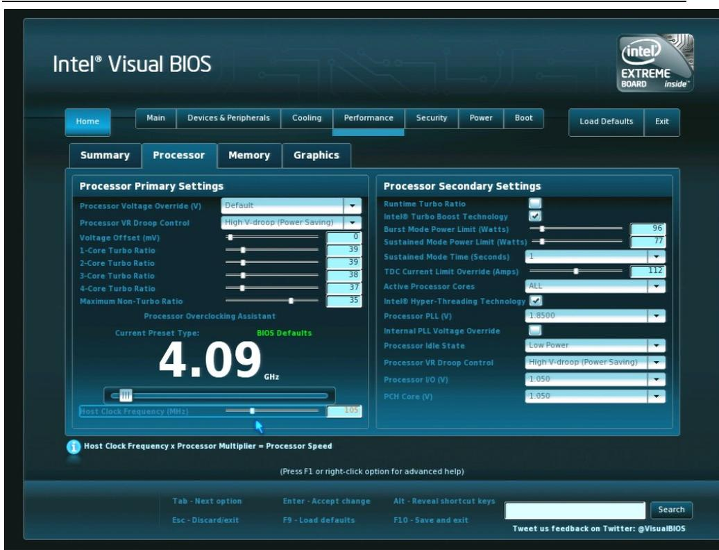
Figure 3.6. BIOS Screen Showing System Clock Frequency Increased to 105 MHz
