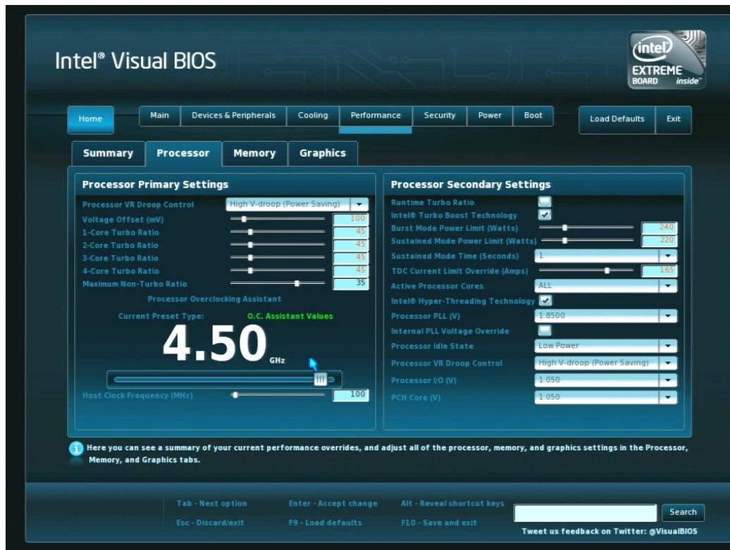
Figure 4.1. 4.5 GHz Processor Speed Using Turbo Ratios
