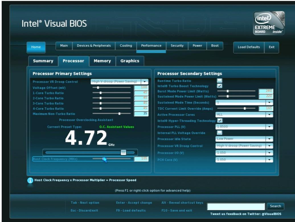
Figure 4.2. 4.72 GHz Processor Speed Using Turbo Ratios with a 105 MHz System Clock Setting
