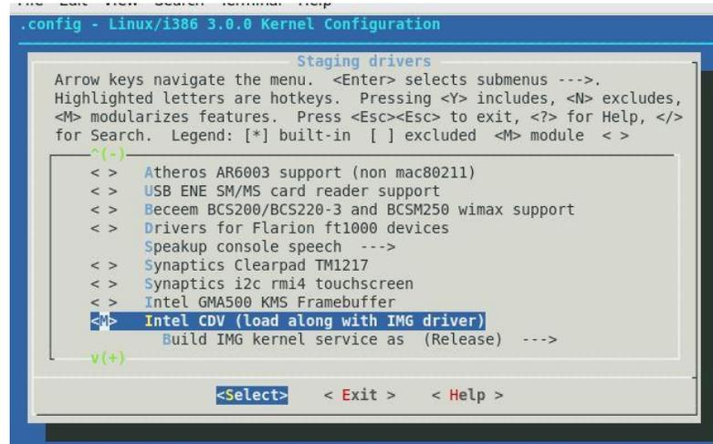
**Figure 3: Menu config Utility - Intel CDV Driver selection**
