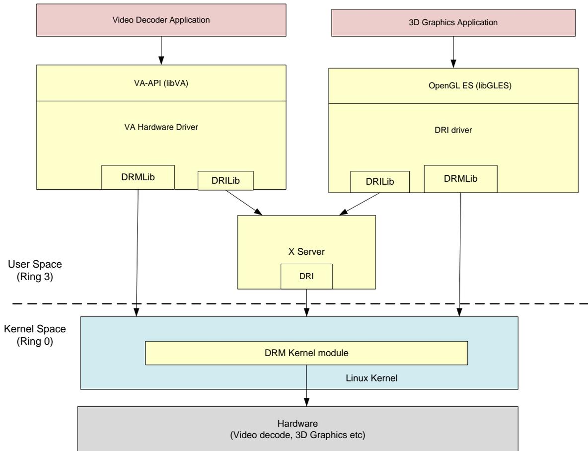
**Figure 1. Overview of Hardware Accelerated Decode**
