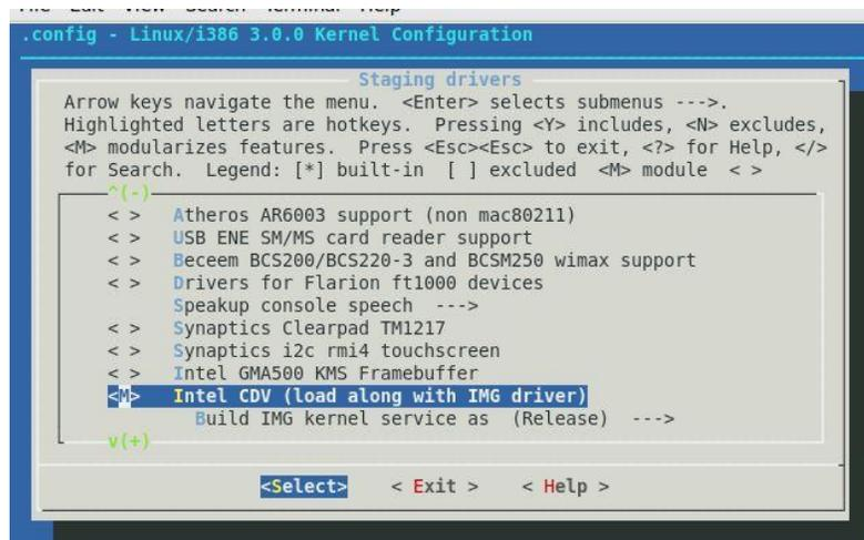
Figure 5: Menu config Utility - Intel CDV Driver selection
