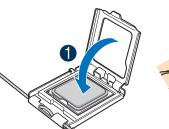
While holding down the load plate, close the socket lever. Ensure that the load plate tab engages under the socket lever when fully closed.
