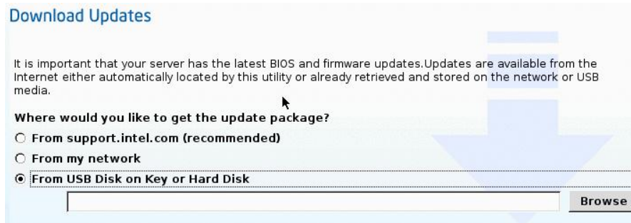
Figure 3-15: Select SUP File in USB Key Folder
