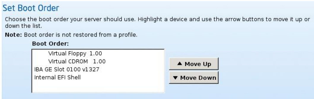
Figure 3-21: Set Boot Order in BIOS Setting
