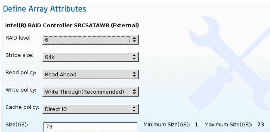
Figure 3-31: Define RAID Array Attributes
