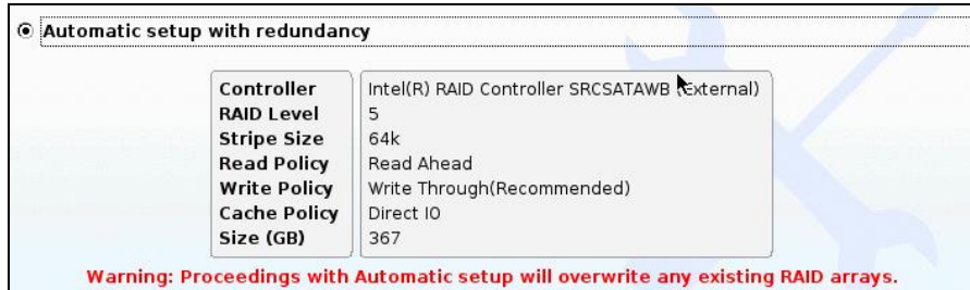
Figure 3-31: Automatic Setup RAID with Redundancy
