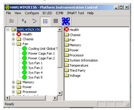
If a fan is installed or reinstalled, PIC sends an alert to the managing console and refreshes the PIC interface, as shown below, reporting the newly installed fan.
