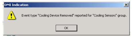
PIC also refreshes the PIC interface so that the removed fan is no longer reported. For example, if the system supports five fans, and Fan 3 is removed, PIC will display status for Fan 1, Fan 2, Fan 4, and Fan 5, with no entry at all for Fan 3.
