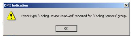
PIC also refreshes the PIC interface so that the removed fan is no longer reported. For example, if the system supports five fans, and Fan 3 is removed, PIC will display status for Fan 1, Fan 2, Fan 4, and Fan 5, with no entry at all for Fan 3.
