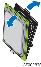
Figure 23. Removing Protective Shipping Cover
