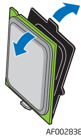
Figure 13. Removing the Processor Protective Cover
