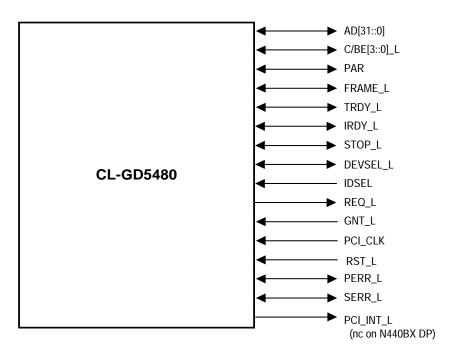
Figure 3-2. Video Controller PCI Signals
