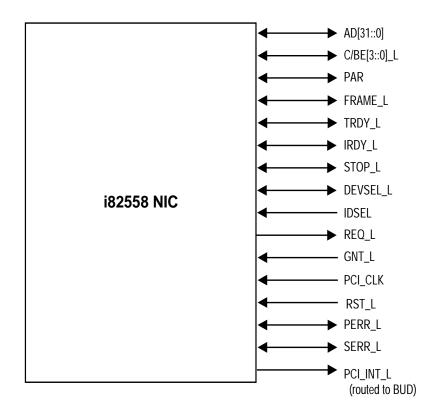
Figure 1-3. Embedded NIC PCI Signals
