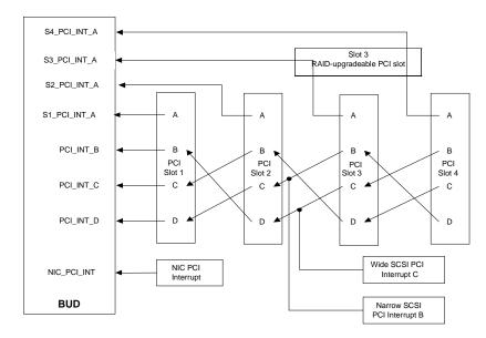
Figure 3-7. PCI Slot Interrupt Swizzle
