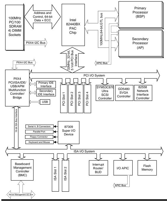
Figure 1.1 N440BX Server Functional Block Architecture
