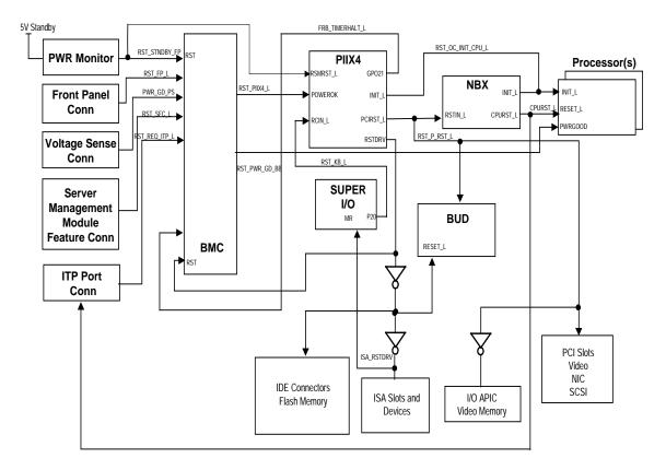
Figure 3-4. Reset Flow Diagram
