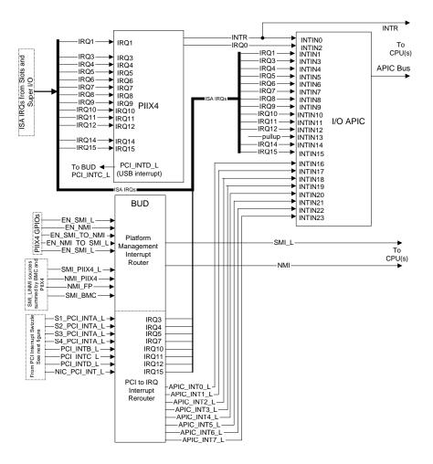
Figure 3-6. Interrupt Structure
