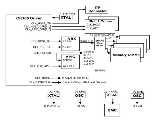
Figure 3-5. Clock Generation and Distribution
