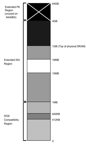
Figure 15. Pentium II/Pentium III processor memory address space
