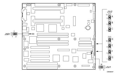
Figure 1.4 N440BX Jumper Connectors
