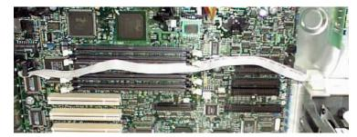
Make sure to stretch the cable that attaches to the drive bay parallel with the DIMM sockets before swinging the SCA hard drive cage into place. Often this cable falls down and can be pinched and damaged when installing the drive bay.
