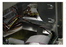
The chassis intrusion sensor connects to the front panel. This is where the reset and power buttons are located. Do not connect the intrusion switch to the N440BX baseboard. When in an Astor Chassis the intrusion sensor is connected to the baseboard.
