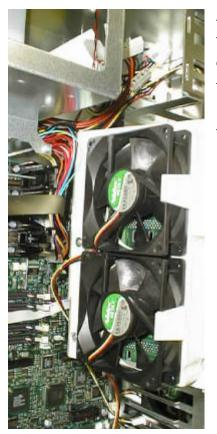
After making sure that the above cable is safe also make sure to pull the wires from the power supply forward so that the plastic fan holder does not cut into the wires. The wires should be in front of the white fan holder when swinging the drive cage into place. In this picture an I/O panel L-cover is being used to gently pull the wires forward while the drive bay is swinging into place.
