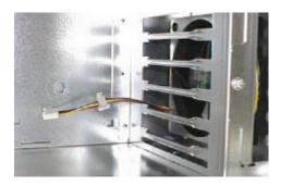
Be sure and notice that there are two connectors on the front fan in the Astor II chassis. The connector on the right is for the N440BX and the connector on the left is for the L440GX.
