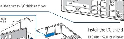
the chassis. A Insert one side edge of shield as shown.
