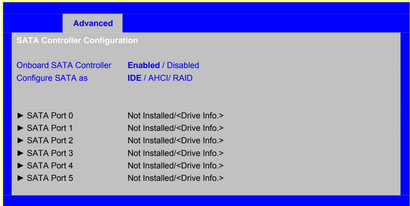
Figure 17. Setup Utility — ATA Controller Configuration Screen Display
