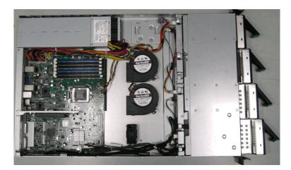
2. Intel® Server System SR1695GPRX (with redundant two AC PSU).
