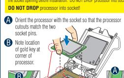
that may damage the socket wires if Processor must align correctly with the socket opening before installation. DO NOT DROP processor into socket!
