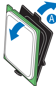
Figure 14. Remove the Processor Protective Cover
