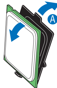
Figure 14. Remove the Processor Protective Cover
