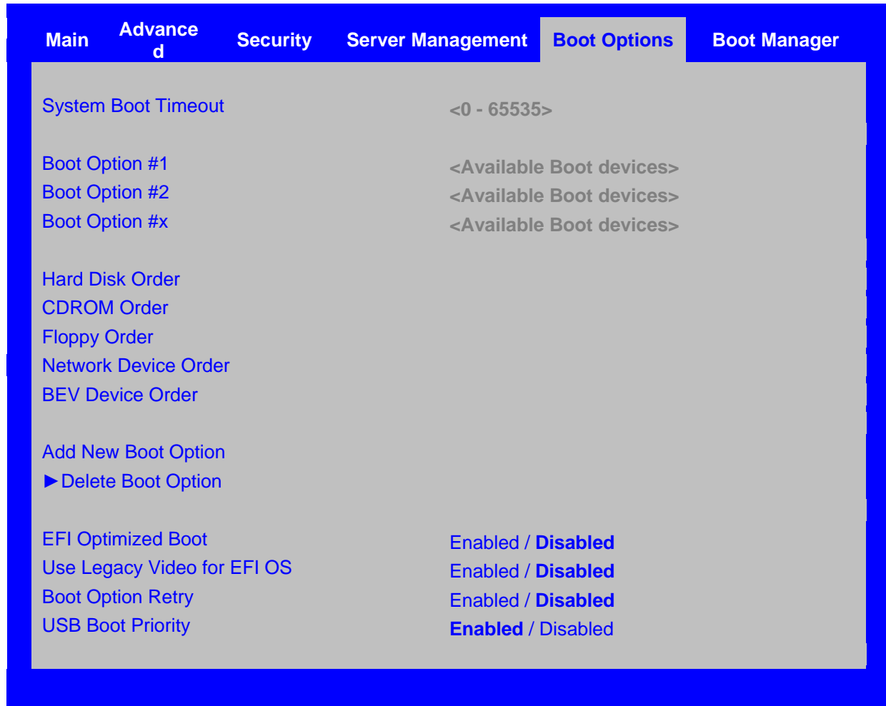
Figure 33. Setup Utility — Boot Options Screen Display
