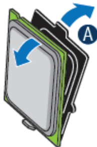
Figure 25. Remove the Processor Protective Cover
