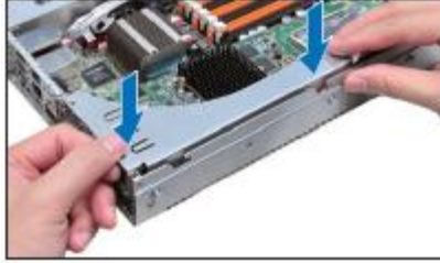
Figure 27. Pressing Rising Card Bracket for Golden Connectors to Fit
