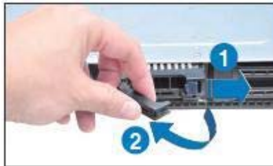
Figure 32. Releasing the Drive Tray
