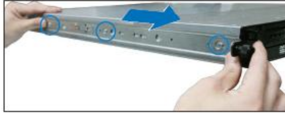
Figure 37. Attaching the Front End of the Server Rail to Side of Chassis
