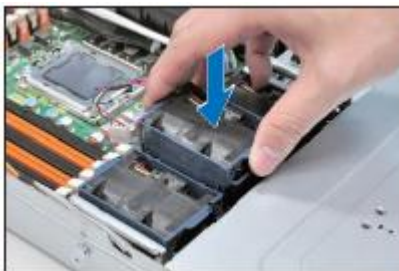
Figure 47. Inserting Fan Into the Fan Cage
