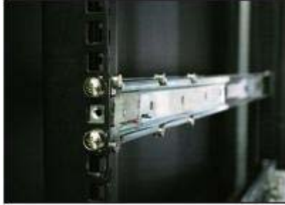
Figure 40. Positioning the Rack Rail to 1U Space on Rack
