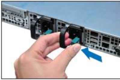
Figure 42. Holding and Pressing the PSU Latch
