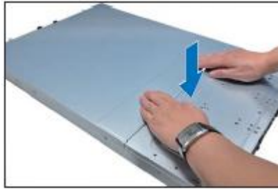
Figure 48. Restoring the Chassis Cover
