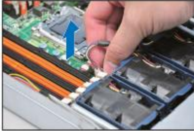
Figure 45. Disconnecting System Fan Cable
