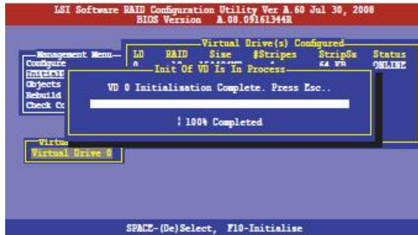
Figure 133. Initialization Progress Bar
