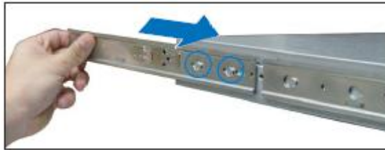
Figure 38. Sliding the Server Rail
