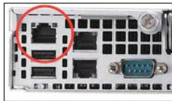
Figure 30. Server Management LAN Port
