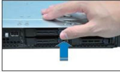
Figure 34. Pushing the Tray Lever
