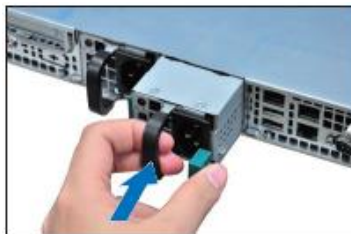
Figure 44. Pushing the New PSU Into the Chassis
