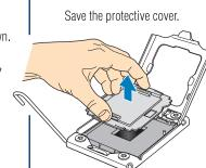
Processor A Grasp the socket protective cover Protective Cover
