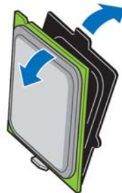
Figure 30. Remove Processor Protective Cover
