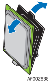
Figure 44. Removing the Processor Protective Cover
