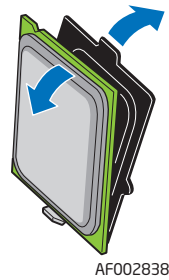
Figure 39. Removing the Processor Protective Cover
