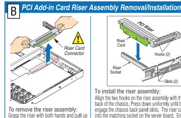
to release riser assembly. Lift straight up.
