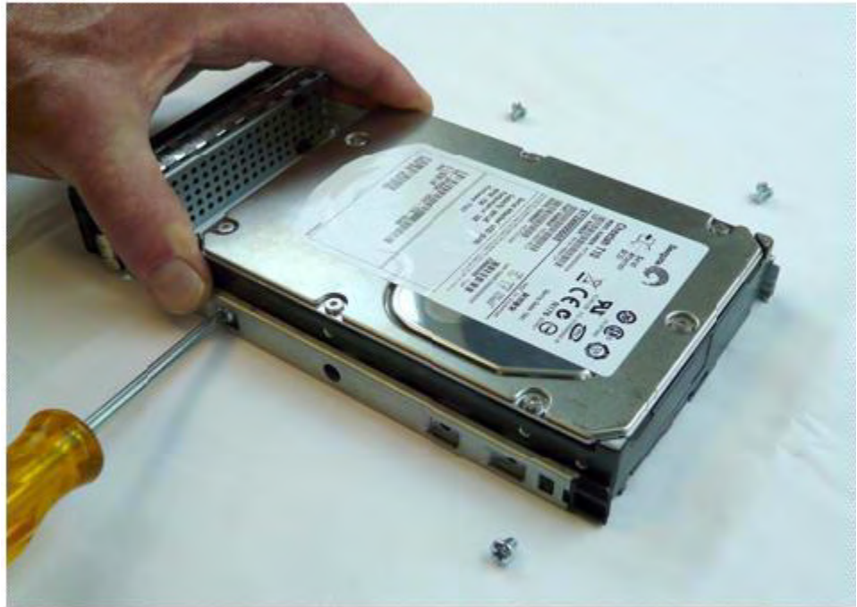
Figure 76. Installing the Four Screws into the Drive Carrier
