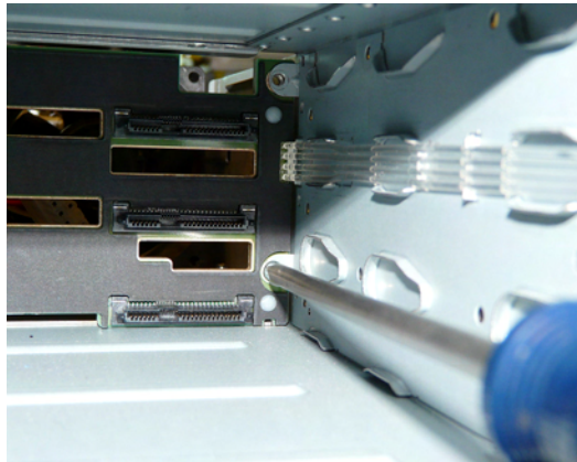
Figure 49. Removing the Screws that Attach the Backplane
