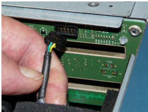
Figure 47. Removing the Logic Cable Connector from the Backplane
