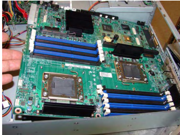
Figure 61. Installing the server board
