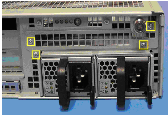
Figure 33. Removing the four screws and cover plate
