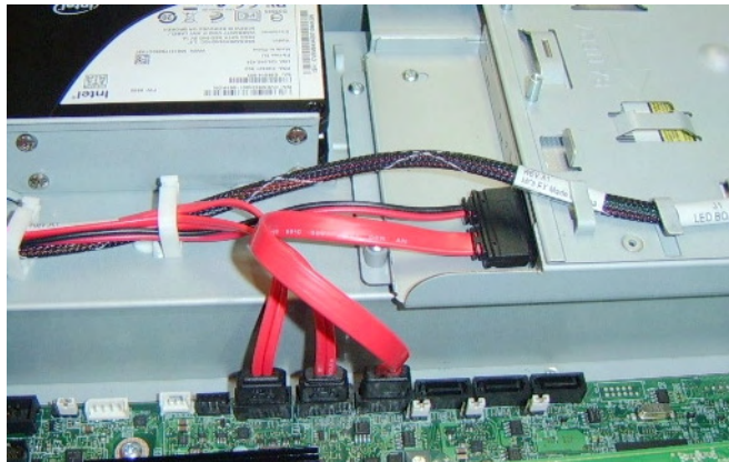
Figure 36. Routing the Cable From the DVD Unit to the Server Board
