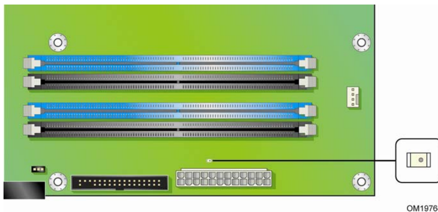
Figure 3. Location of Standby Power Indicator
