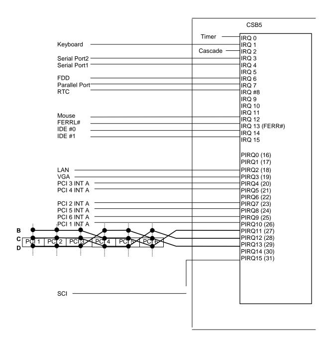
Figure 5. SAI2 Baseboard Interrupt Routing Diagram (Symmetric Mode)
