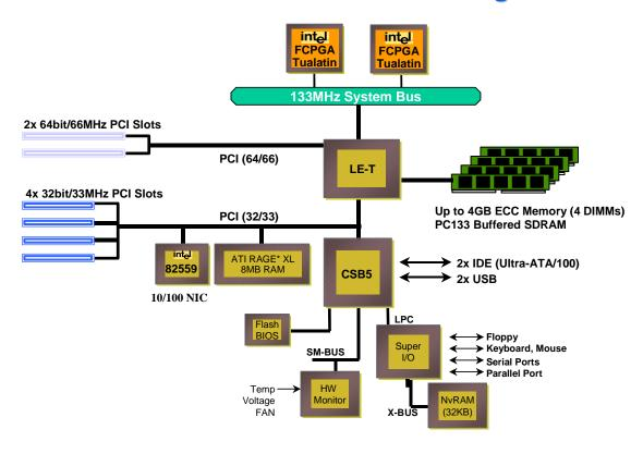
Figure 1. SAI2 Server Board Block Diagram
