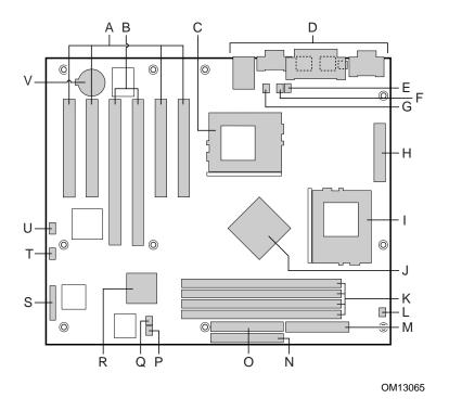
Figure 6. SAI2 Server Board Jumper and Connector Locations
