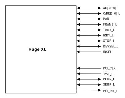
Figure 3. Video Controller PCI Signals
