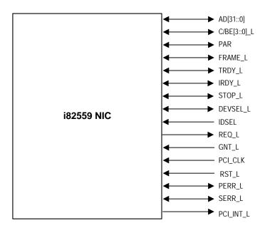
Figure 2. Embedded NIC PCI Signals
