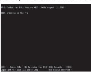
When Intel® RAID BIOS Console 2 starts, it will display the Intel® RAID Controller SASMF8I installed in the system. Click on the "Adapter No." radio button,
