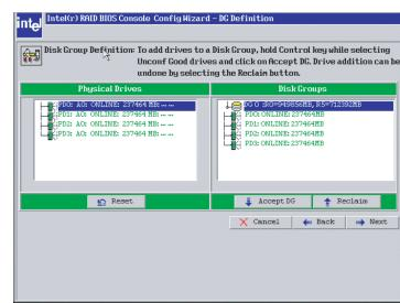
Select the **RAID Level** from the pull-down box. Select the **Stripe Size.** Enter the size of the logical drive. Click **Accept.** Click **Next** if the program does not automatically progress to the next screen.
