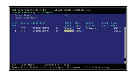
When the RAID Disk status is listed as shown below, press <**C**> to create an array.
