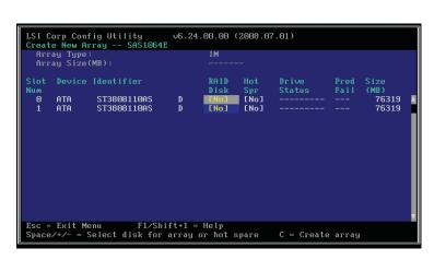
Press <M> to keep existing data, or press <**D**> to overwrite existing data.
