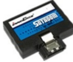
Figure 41. Innodisk* SATA Disk-on-Module (DOM) device
