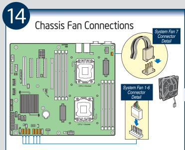
For a non-Intel server chassis, see the documentation accompanying your chassis for specific chassis fan connection requirements. Refer to the "Making Connections to the Server Board - Quick Reference"
