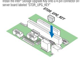
♦ Note: The server board is capable of supporting additional chipset embedded SAS and RAID options from the SCU controller when configured with one of several available Intel® RAID C600 Upgrade Keys, See Product Specification for the varies of options that different keys support.
