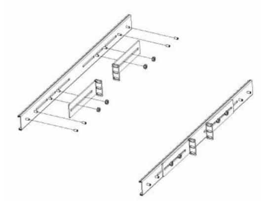
3. Install the two outer rail subassemblies in the rack using twelve 10-32x1/2" SEMS screws or whatever rack hardware is necessary.
