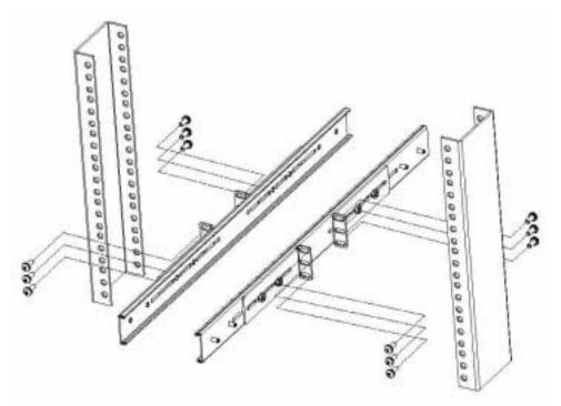
4. Slide the system into the rack making sure the inner rail is 'dovetailed' with outer rail.
