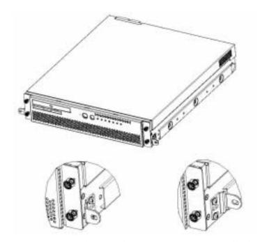
3. Using the 4 outer studs, assemble the mounting brackets to the outer rail with four 8-32 KEPS nuts. Insert 4 thread covers over the 4 inner studs.
