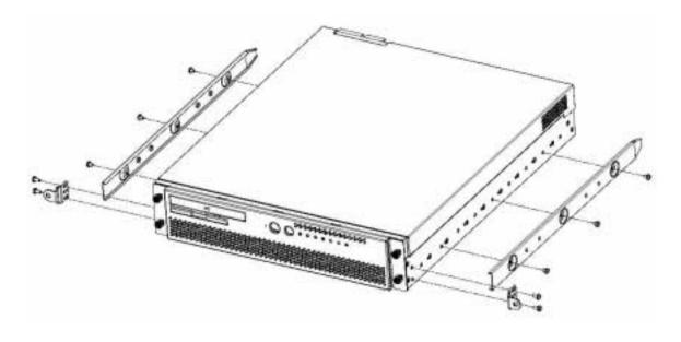
2. Attach the front-tab mounting bracket to the chassis with two 8-32x1/4" SEMS screws (both sides).
