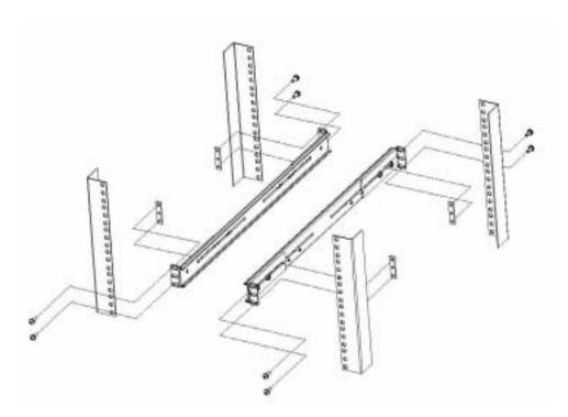
5. Slide the system into the rack making sure the inner rail is 'dovetailed' with outer rail.
