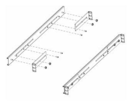
4. Install the two outer rail subassemblies in the rack using eight 10-32x1/2" SEMS screws (use four bar-nuts if necessary).
