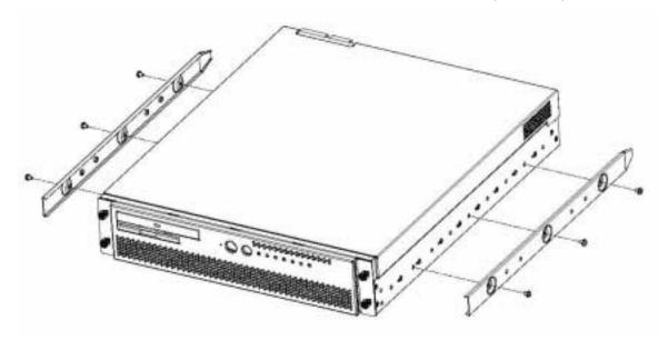
2. Using the four inner studs, assemble the mounting brackets to the outer rail with four 8-32 KEPS nuts. Insert four thread covers over the four outer studs (two times).
