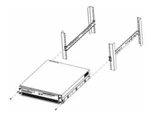
$6. \quad In stall \ two \ 10\text{--}32X1/2" \ SEMS \ screws \ to \ hold \ the \ front-tab \ mounting \ bracket \ to \ the \ rail.$
