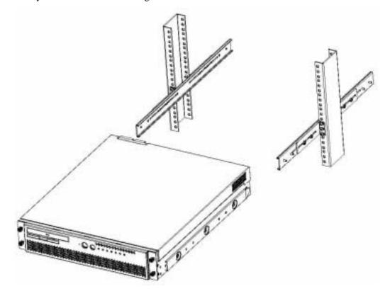
5. Install four 8-32x7/16" SEMS screws through the clearance slots in the side of the outer rail assembly into the inner rail (two sides).
