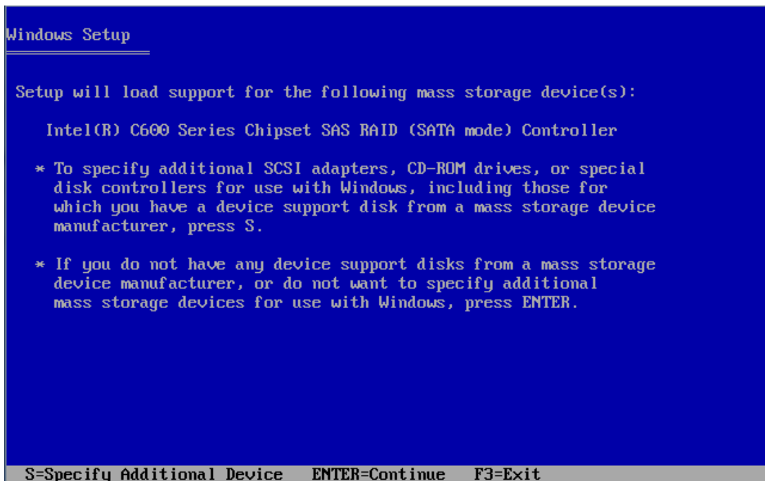
Figure 45. Load Support for Mass Storage Device
