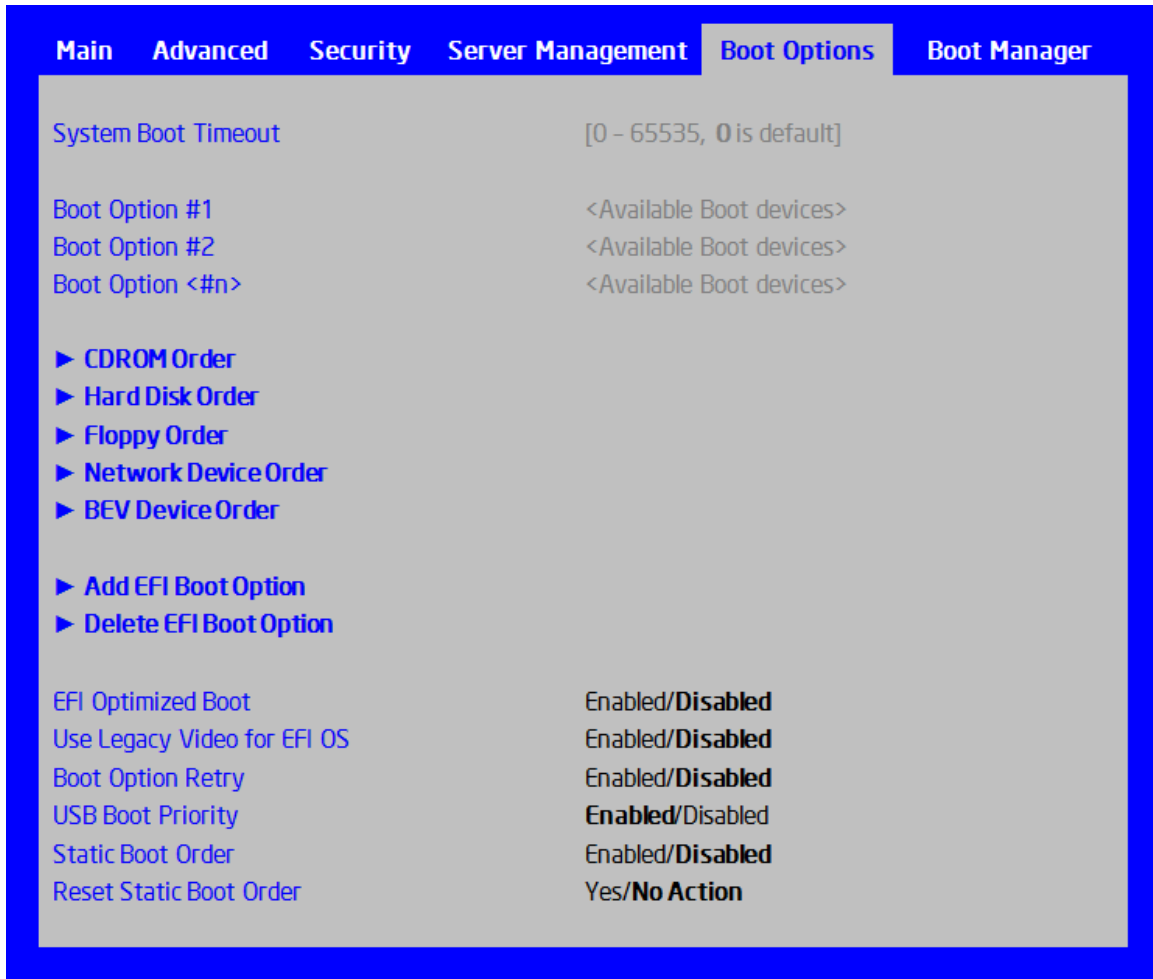
Figure 36. Boot Option Screen
