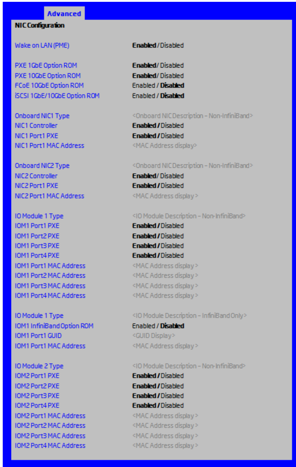
Figure 26. NIC Configuration Screen
