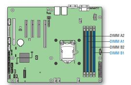
Memory Type: Minimum of one 1 GB, DDR3 1066/1333 MHz ECC UDIMM. Note: For additional memory configurations, see the Techinical Product Specification on the Intel® Server Deployment Toolkit CD that accompanied your Intel® Server Board S1200BTL, or go to:
