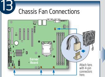
For a non-Intel server chassis, see the "Making Connections ... Quick Reference" section below, and the documentation accompanying your chassis for specific chassis fan connection requirements.
