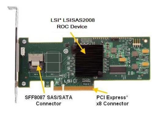
Figure 4 Intel® RAID Controller RS2WC040 Physical Layout
