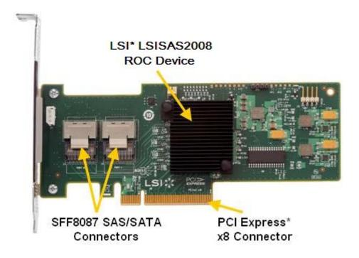
Figure 2 Intel<sup>®</sup> RAID Controller RS2WC080 Physical Layout
