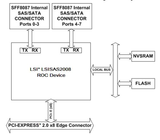
Figure 1 Intel® RAID Controller RS2WC080 Hardware Block Diagram
