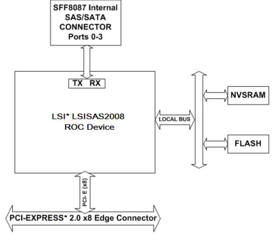
Figure 3 Intel® RAID Controller RS2WC040 Hardware Block Diagram
