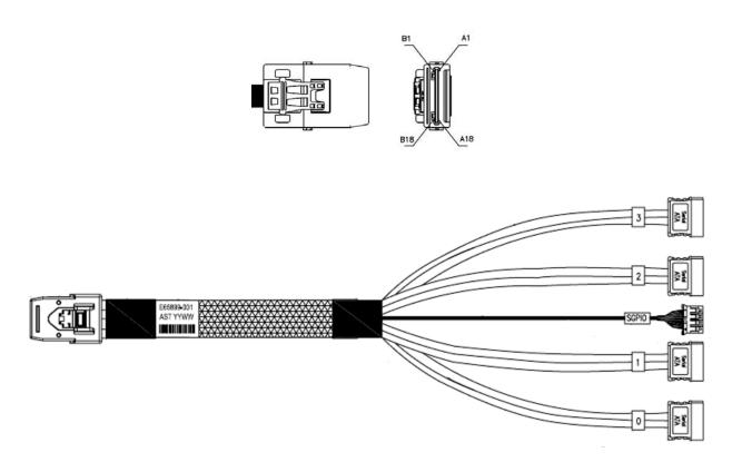
Figure 6 SFF8087 to Four-port Internal Cable with one SGPIO Connector
