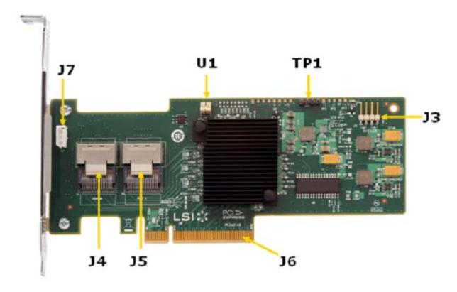
**Figure 7 Jumpers and Connectors**
