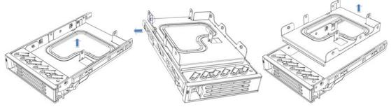
Figure 2. Removing the Bracket from Carrier
