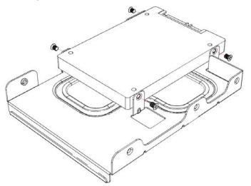
Figure 4. Securing screws on the bracket
