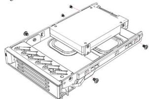
Figure 6. Securing Screws on the Rails
