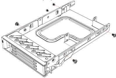
Figure 1. Removing Screws from Rail and Adaptor Plate
