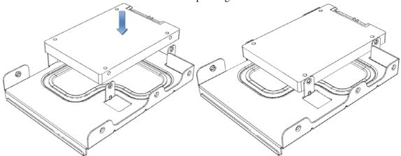
Figure 3. Installing 2.5" HDD into the bracket
