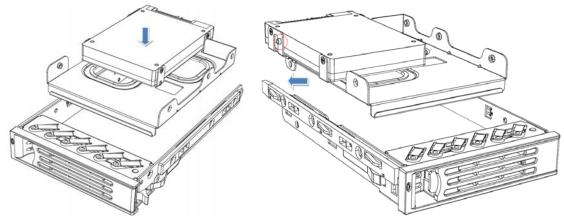
Figure 5. Installing the bracket into the rail
