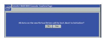
2 Select **Fast Initialize** to do a preliminary initialization of the drives for loading the operating system. A full initialization will occur in the background.
