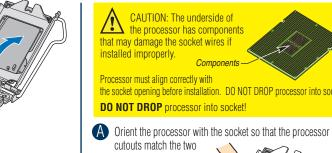
socket pins. B Note location of gold key at corner of processor.
