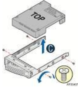
Figure 83. Installing Hard Disk Drive – Removing 3.5" HDD interface bracket
