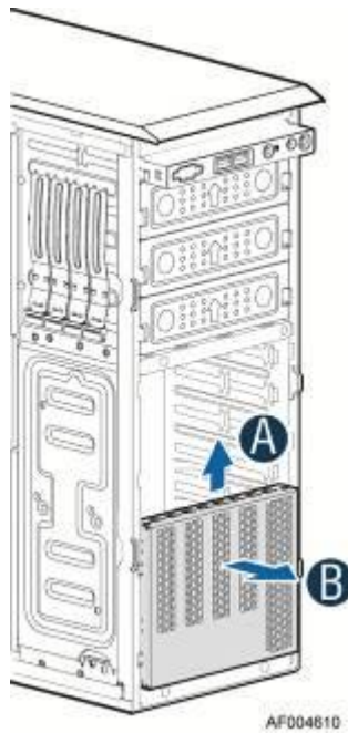
Figure 72. Removing the Hot-swap HDD EMI Shield
