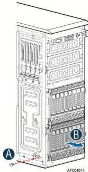
Figure 74. Removing the bottom 8x2.5" Hot-swap HDD Cage Assembly
