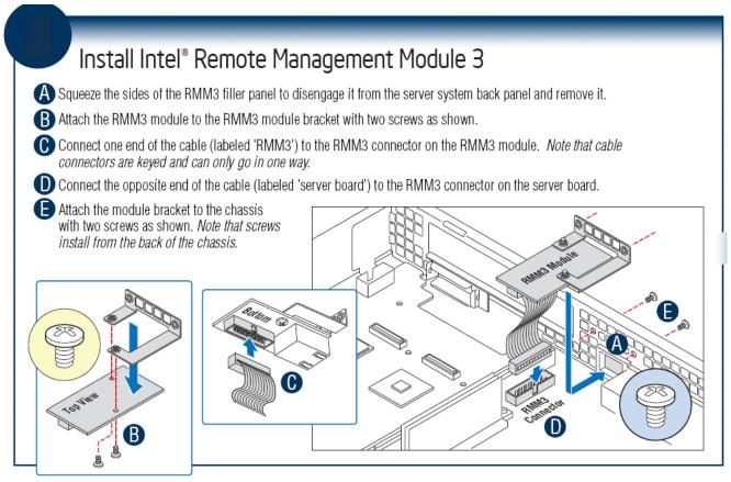
Figure 4 – Installing Intel<sup>®</sup> RMM3 on Intel<sup>®</sup> Server Boards S5500UR and S5500WB
