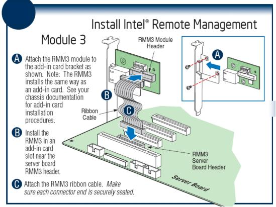
Figure 5 – Installing Intel<sup>®</sup> RMM3 on Intel<sup>®</sup> Server Boards S5520HC, S5520BC, and S5520SC
