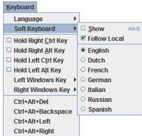
Figure 29: Remote Console Keyboard Soft Keyboard Sub Menu
